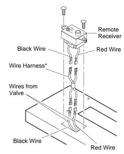
Figure 29 - Installing Remote Receiver
